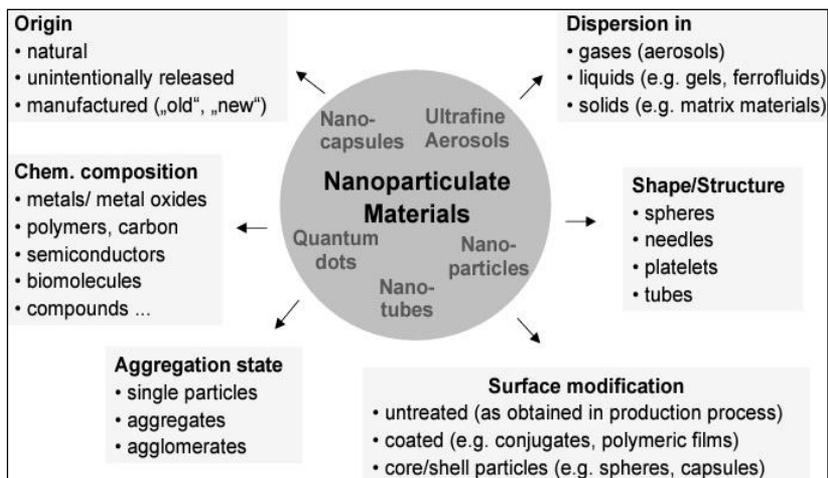
**Fig:** Characteration parameters of nanoparticulate materials (source; Luther, 2004).
