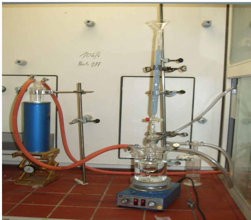
Fig 4. The Constructed Modified Jones Reductor
